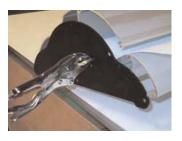
3. Position the left-hand end plate onto the system so that the flat metal bar of the reel protrudes from the slot in the end cap. Grip the flat bar with a vice grip.
