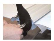
4. Rotate the flat bar clockwise. The table above indicates the number of rotations required for different size BannerBug® models.
